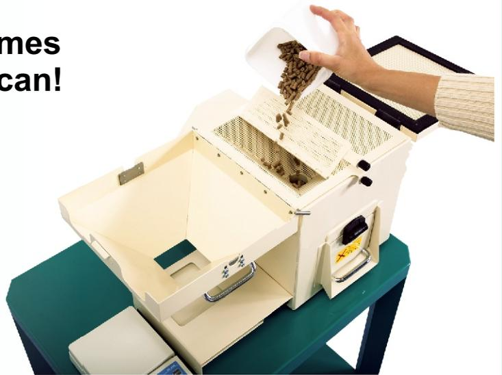
Simulates the pellets transportation environment from mill to trough.
